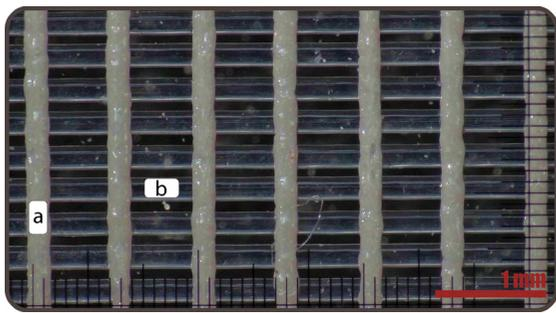
Figure 6: Printed samples – PLA and TPU f-fibre (macro photo): (A) TPU material with high porosity issues; (B) PLA (transparent) material
