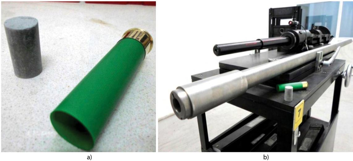
Figure 3: Ammunition – compressed iron powder (a) and barrel used in BSP tests (b)
