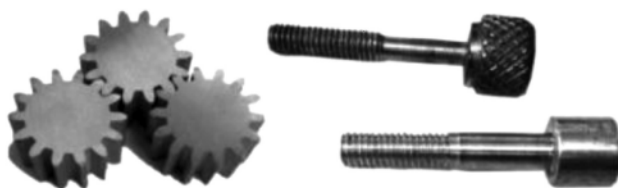
Figure 1: Fabricated gears and screws of 5 φ/1% B 4 C/AA6061 chips at SMART-AMMC, UTHM
