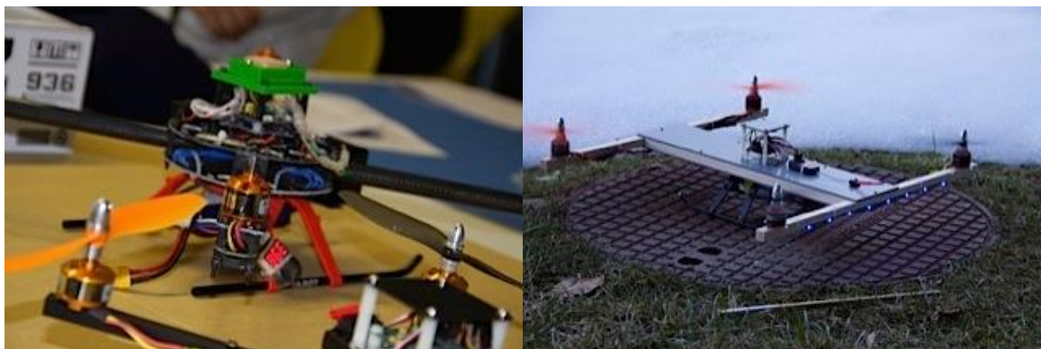
Picture 3: Two built models of the quadcopter. The first one made out of aluminum using a set, the second one built from scratch using wood. Both were built during the pilot workshop in Bad Hofgastein, Salzburg, Austria.
