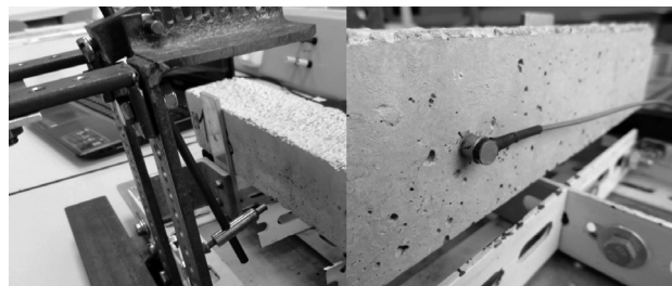
Figure 2: Images of measurement with the Impact-Echo method Slika 2: Posnetka merjenja z metodo odmeva zvočnih valov
