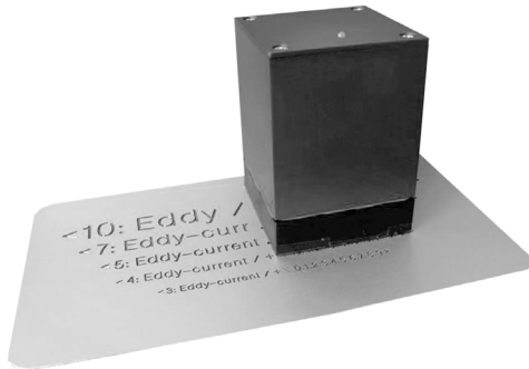
Fig. 26. The flat array on the engraved aluminium sheet for testing the spatial resolution
