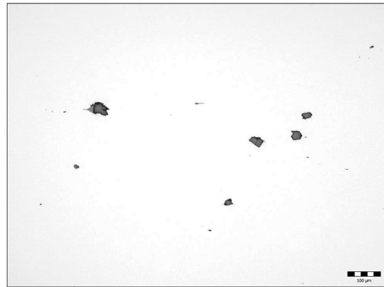
Figure 9: Non-metallic inclusions in the piece forged from Melt 2. Magnified 65×.
