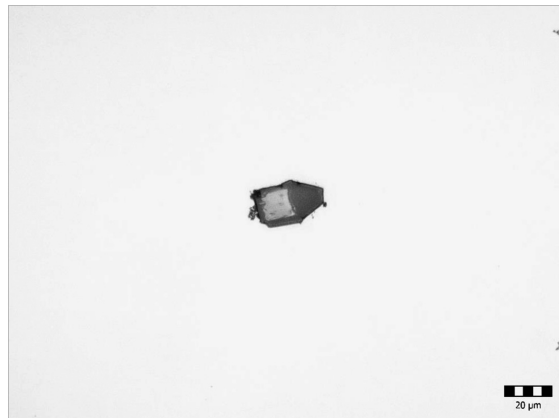
Figure 10: Non-metallic inclusions in the piece forged from Melt 2. Magnified 330×.
