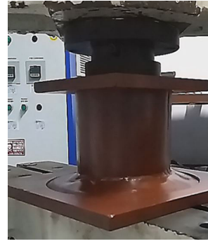
Fig. 14. PPS specimen after collapse
