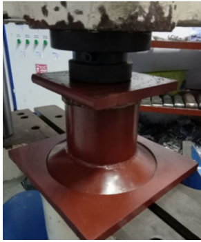
Fig. 13. PPS specimen before collapse
