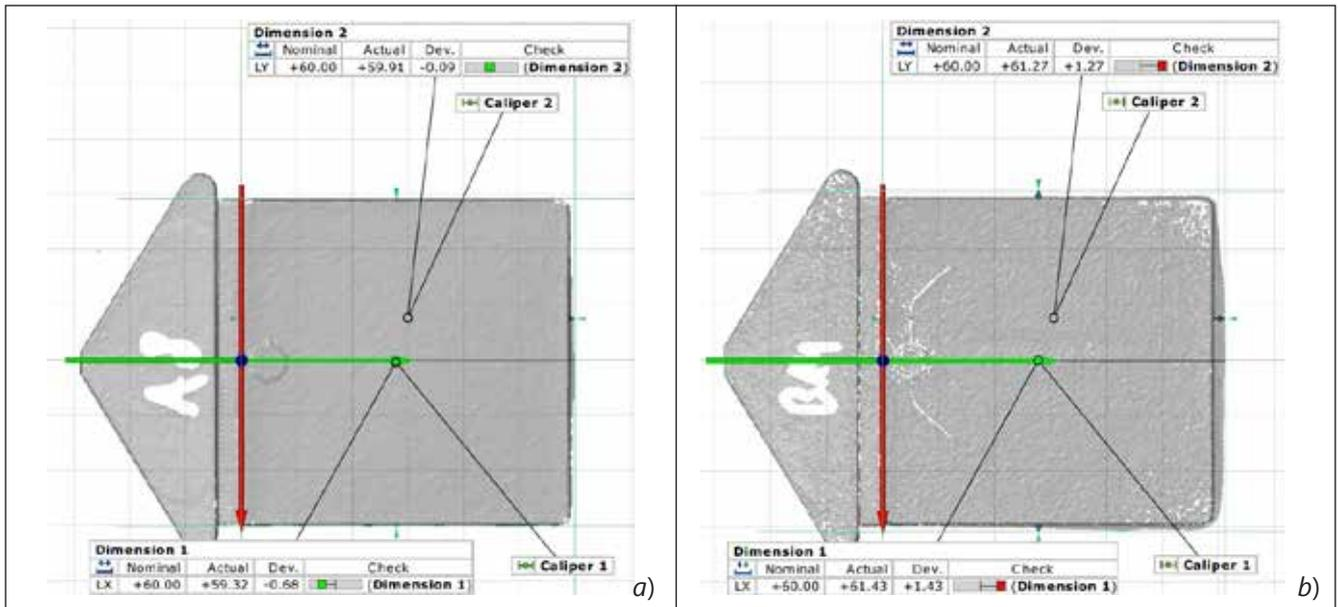
**Figure 4.** Scanned test specimens (a) specimen 8 produced on a new tool steel insert, (b) specimen 14 produced on a tool steel insert with visible signs of a macro-crack.
