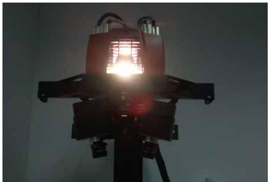
**Figure 3.** Optical 3D digitizer ATOS II SO with two high-resolution CCD cameras
