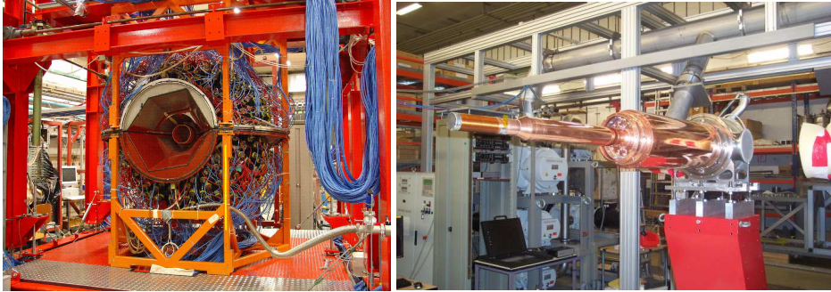
Fig. 1. Crystal-Ball detector at MAMI and the horizontal cryostat of the frozen spin target, which keeps temperatures of about 20mK.
