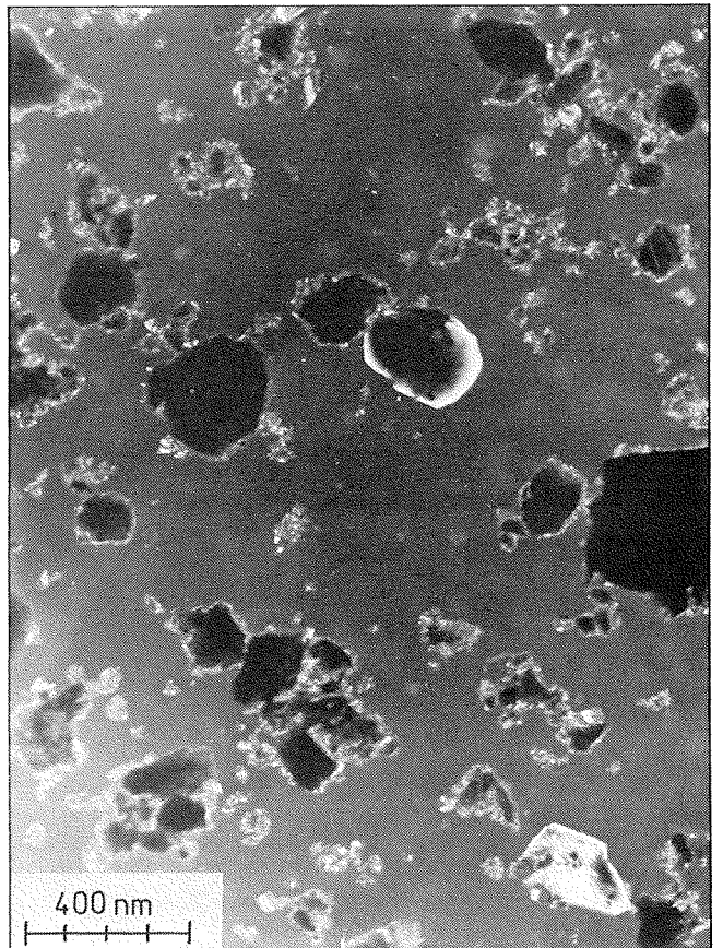
Fig. 6: Micrograph of \text{RuO}_2 powder prepared by ruthenium oxidation at 1,000^\circ\text{C} (ground for 40 hours).
