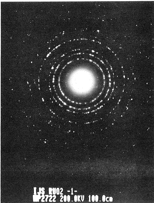
Fig. 4b: Electron diffraction pattern from \text{RuO}_2 powder (type Ru-109 by Shoe Chem. Inc.).
