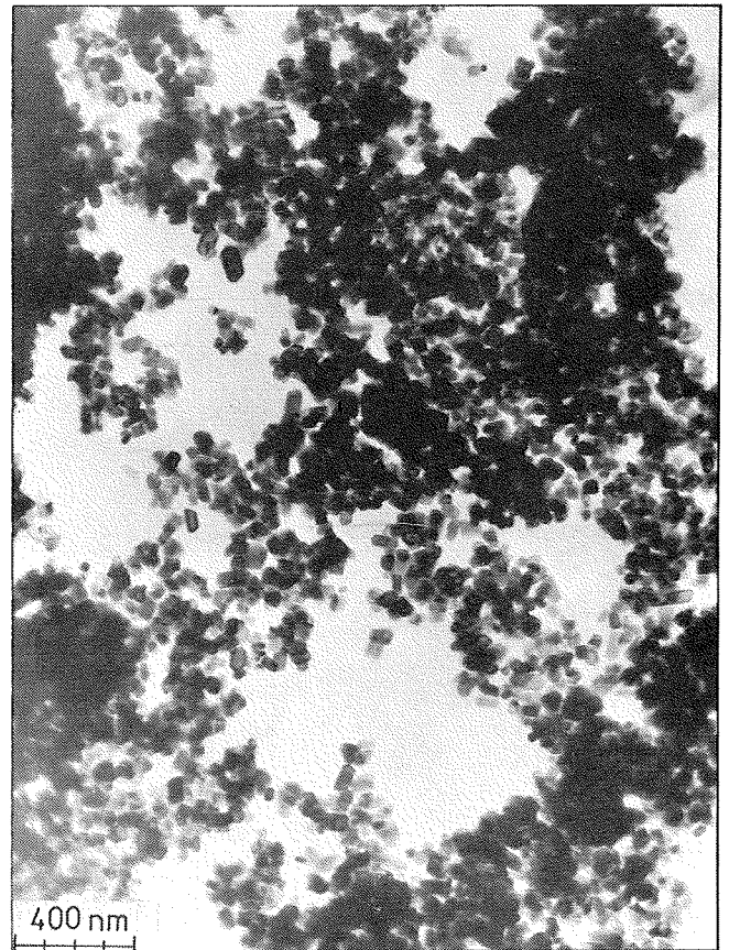
Fig. 5: Micrograph of \text{RuO}_2 powder of type Ru-109 shows perfectly created microrystalline grains without clusters and conglomerates.
