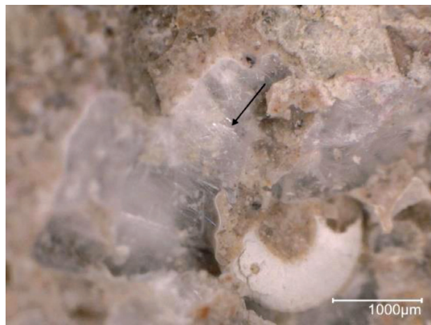
Figure 4: 3D rendering of the ettringite crystals in the pores
