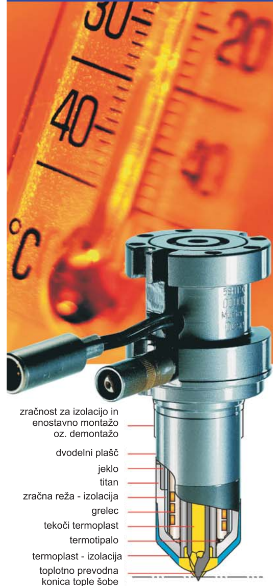
Slika 3: HPS-AT-polž (High performance screw - avtomotive) [1]
