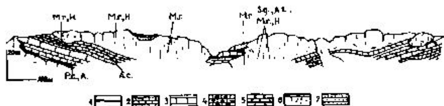
Fig. 3. Jurassic coralligenous limestone and associated sediments exposed in the axis of syncline at north of Topalu (Central Dobrogea); 1 marls; 2 well bedded pelitic limestone; 3 thick bedded limestone with organic detritus; 4 limestone with cherts; 5 dolomitic limestone; 6 coralligenous limestone; 7 glauconitic sandstone (cretaceous); Ammonite fauna: P.c. = Physodoceras contemporaneum (Favre) A.c. = Aspidoceras cyclotum Neum; A. = Atarioceras ; Hydrozoan fauna: M.r. = Milleporidium remesi Stein.; H. = Hudsonella n. sp.; S. g. = Spongiomorpha aff. globosa Yabe & Sugiyama; A.L. = Actinostromaria tokadiensis Yabe & Sugiyama
