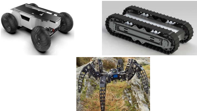
Figure 2: Some of possible traction methods applicable for Agriculture robots
