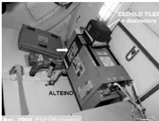
Figure 7: The detector ALTEINO on the ISS during the ENEIDE mission in 2005. On top of the active detector it is visible a blue bag containing polyethylene, Kevlar; and Nextel shield blocks, and passive TLD detectors (ESCHILO tiles). Photo from Spillantini et al. (2007), courtesy of Dr. Marco Casolino (INFN, Rome, Italy).
