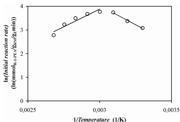
Figure 10. Arrhenius Plot for Acylation of ( R,S )-1-phenylethanol with Vinyl Acetate in [bmim][BF 4 ], Catalyzed with Immobilized CALB.
