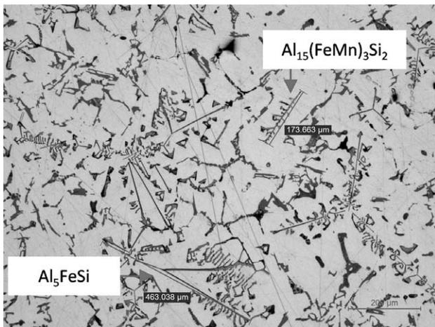
**Figure 2:** Light micrograph of the sample from melt no. 2 with indicated measurements of iron-based phases
