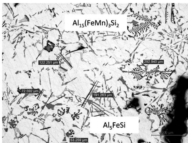
**Figure 1:** Light micrograph of the sample from melt no. 1 with indicated measurements of iron-based phases
