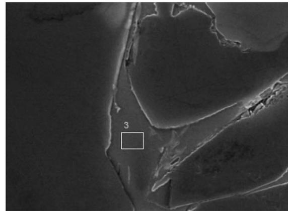
**Figure 4:** SEM micrograph of the sample from melt no. 3 with indicated EDX measurement of iron-based α-phase (chemical composition in mass fractions: w(Al) = 59.31 %, w(Si) = 9.25 %, w(Cr) = 13.71 %, w(Mn) = 5.03 %, w(Fe) = 11.17 %, w(Cu) = 1.54 %)
