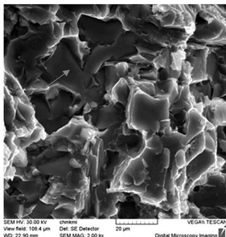
**Figure 6:** SEM micrograph of the sample from melt no. 3 with indicated EDX measurement of fracture area of tensile-test specimen (chemical composition in mass fractions:  $w(\text{Al}) = 56.57\%$ ,  $w(\text{Si}) = 8.77\%$ ,  $w(\text{Cr}) = 17.28\%$ ,  $w(\text{Mn}) = 5.72\%$ ,  $w(\text{Fe}) = 11.67\%$ )
