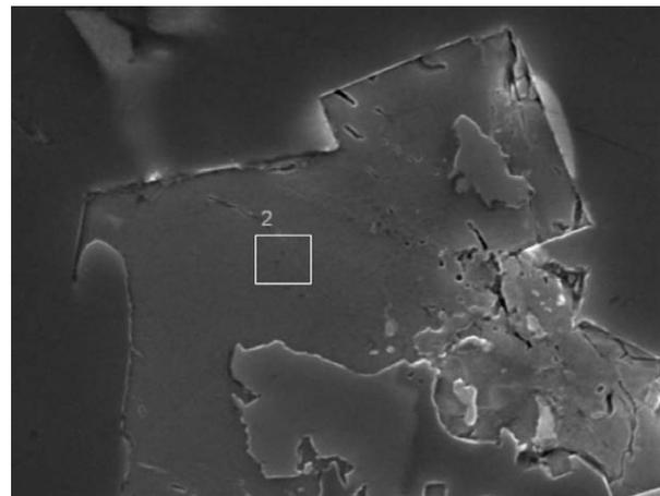
**Figure 5:** SEM micrograph of the sample from melt no. 3 with indicated EDX measurement of sludge particles (chemical composition in mass fractions: w(Al) = 50.13 %, w(Si) = 9.14 %, w(Cr) = 18.37 %, w(Mn) = 6.68 %, w(Fe) = 13.81 %, w(Cu) = 1.87 %)
