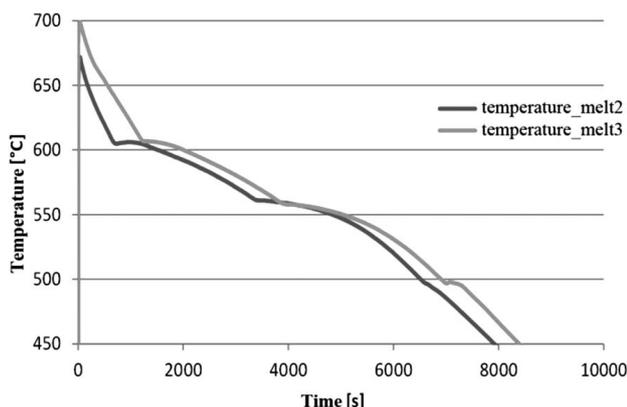
**Figure 7:** Cooling curves of melts 2 and 3 after the additions of various amounts of master alloy AlCr20
