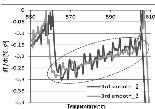
**Figure 8:** Comparison of first derivations in the area of segregation of iron-based phases from melts no. 2 and 3
