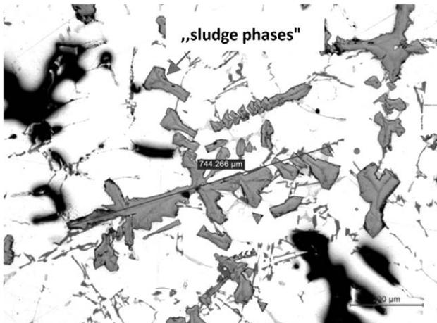
**Figure 3:** Light micrograph of the sample from melt no. 3 with indicated measurements of iron-based phases
