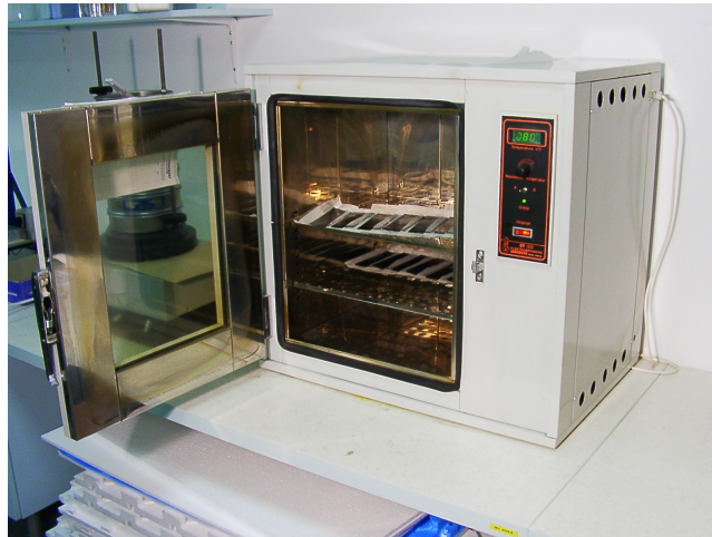
Slika 4: Pečica – sušilnik ELEKTROMEHANIKA LABONOVA ST 80 Figure 4: Oven – Dryer ELEKTROMEHANIKA LABONOVA ST 80
