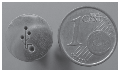
Sl. 4. Elektroda za PPME, izdelana z VC Fig. 4. MEDM electrode machined with WJ technology
