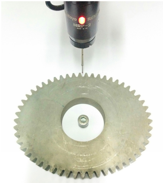
Fig. 18. Validation of the algorithm with a coordinate measuring machine
