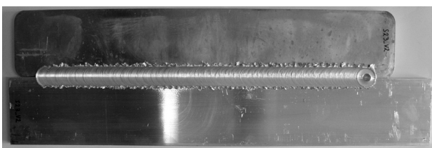
Figure 5: Plates joint with FSW (upper plate of AA413.0 alloy, lower plate of AA1050 alloy)
