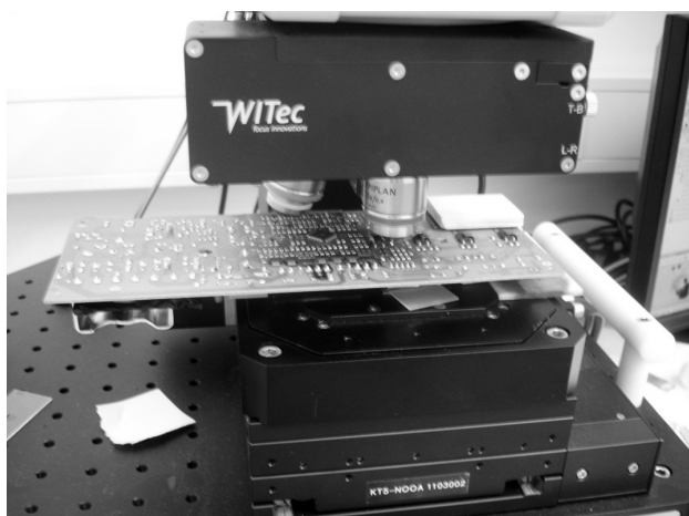
Figure 5: Measurement of the Raman spectra on the uncoated and coated EB substrate
