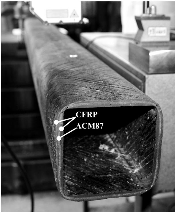
Figure 3: Cantilever square tube consisting of K63712 CFRP and the ACM87 cork-rubber composite material: sample C
