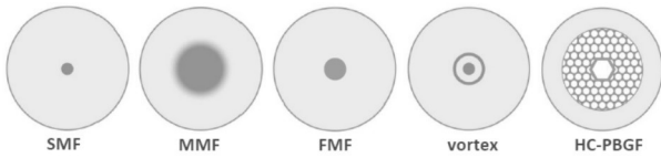
Figure 4: Single-mode fiber (SMF), multi-mode fiber (MMF), few-mode fiber (FMF), vortex fiber, hollow-core photonic band-gap fiber (HC-PBGF).
