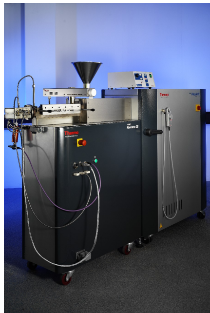
Fig. 8. The PolyLab OS laboratory twin-screw co-rotational extruder (Thermo HAAKE Electron Corporation), consisting of A – RheoDrive 4 and B – Rheomex PTW 16
