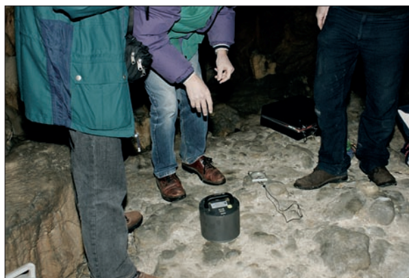
Fig. 3: Accelerometer installation at Velika Gora chamber in 2010 (Photo: S. Šebela).
