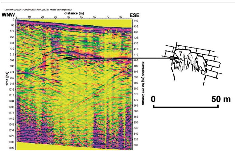
Fig. 4: GPR profile P2 and cross-section of Pretnerjeva Dvorana by Gospodarič (1985). The arrow marks the corresponding trigonometric point.
