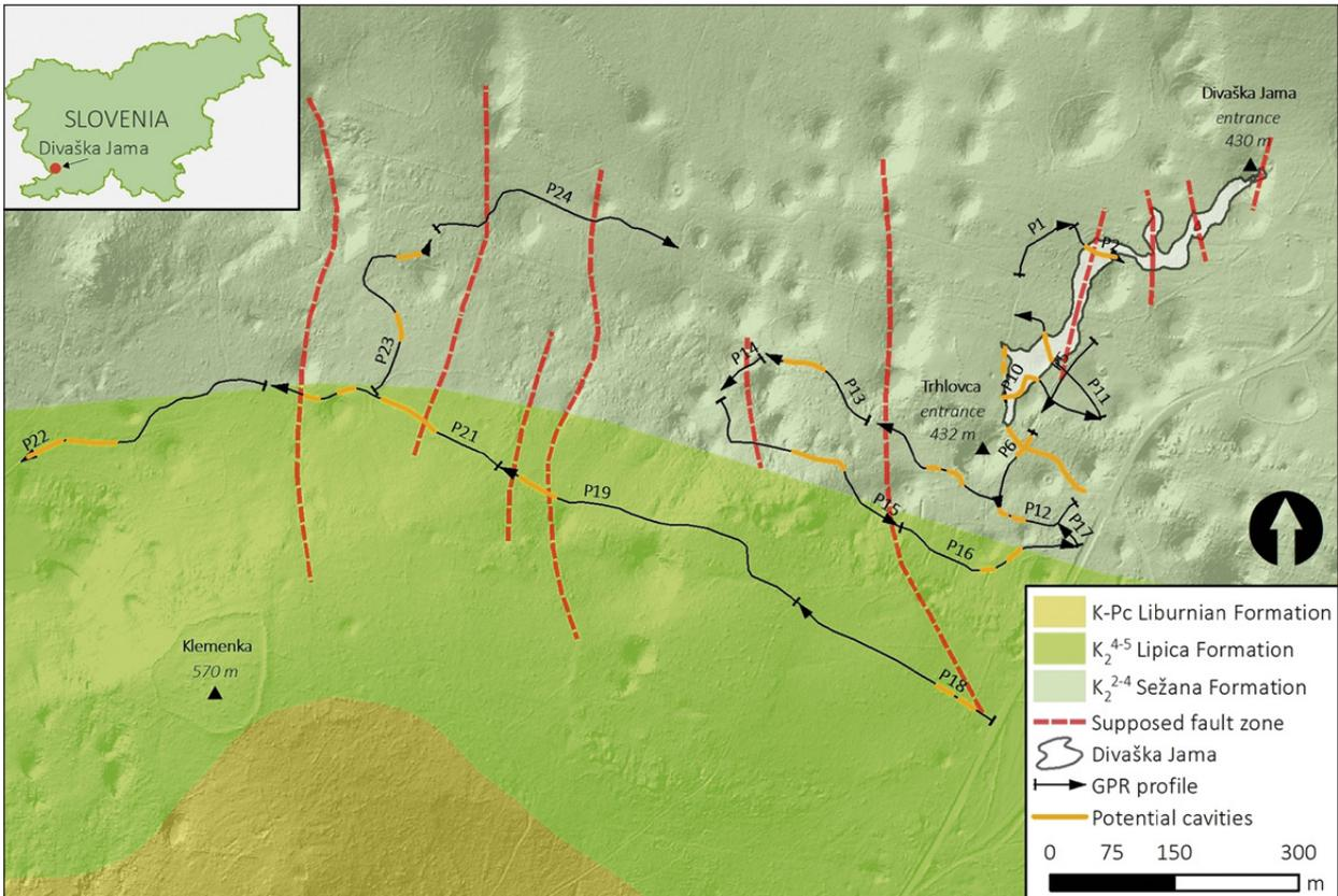
Fig. 23: Lidar map (source ARSO 2017) with GPR “Roteg” profiles (black), tectonics (violet), layers (green and grey) and detected large cavities (orange). Geology after Jurkovšek et al. 1996.
