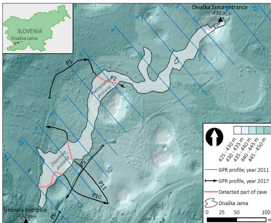
Fig. 1: GPR profiles measured above known part of the cave Divaška Jama. Blue lines – profiles of Gosar (2012), black curves – profiles of “Rotež” GPR 2017. Red – detected ceiling of the cave (Figs. 4, 7 and 8).
