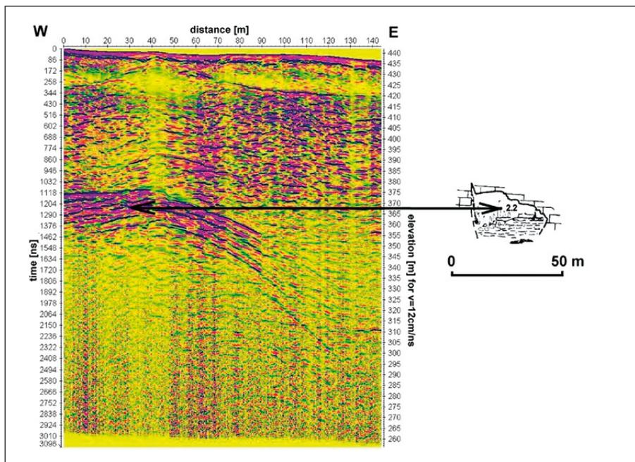
Fig. 7: GPR profile P10 and cross-section of Žibernova Dvorana by Gospodarič (1985). The arrow marks the corresponding trigonometric point.
