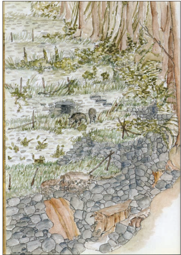
Figure 6: First phase of abandonment: Development of parasitic vegetation, expanding to the wood. Slow erosion of the foundation. The last consequences of the abandonment caused by river's erosion, no long under control, are the destructive landslides.
