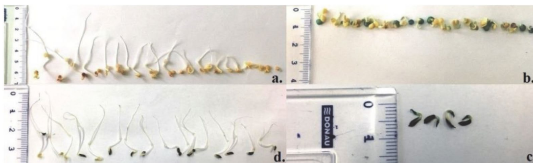
Figure 6. Mustard (a, b) and lettuce (c, d) seeds before (a, d) and after (b, c) seed growth test
