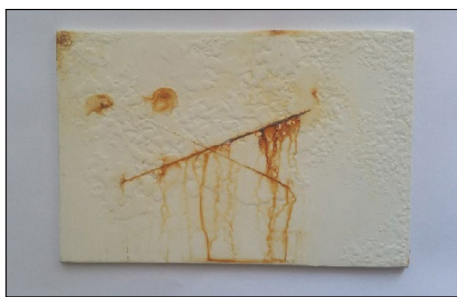
Figure 5. PA7 after 1000h under the salt spray test before adding more adhesion promoter and surface agent.
