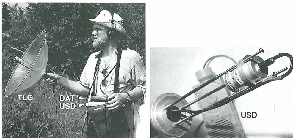
Fig. 2: A recordist with ultrasonic equipment used in the field survey of T. brullei . Left: TLG - Telinga parabola with ultrasonic microphone, DAT - digital tape recorder, USD - ultrasonic ("bat") detector; right: details of the attachment of the ultrasonic microphone in the reverse position to the Telinga parabola, in the background the bat detector S-25, Ultra Sound Advice.
