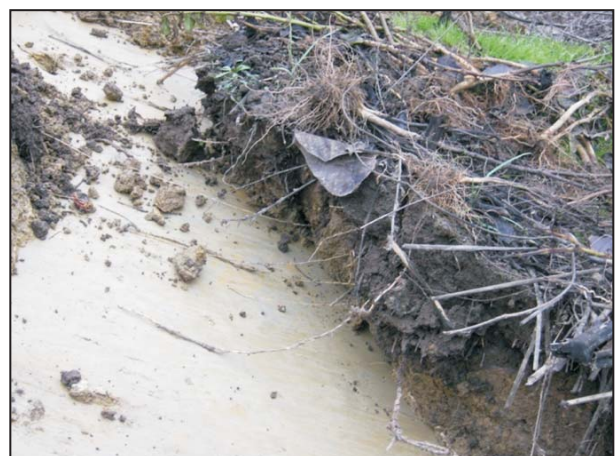
Figure 12. Revealed surface of rupture after the landslide reactivation in December 2009.
