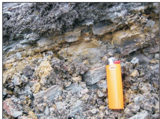
Figure 9. Detail of distorted structure of marlstones in the left side scarp (photo December 2009).
