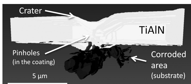
Figure 3: 3D reconstruction of a corrosion volume under a TiAlN coating on a site where a crater with pin holes was present Slika 3: 3D-rekonstrukcija korodiranega območja pod TiAlN-prevleko na mestu, kjer se je nahajal krater s "pinholi"
