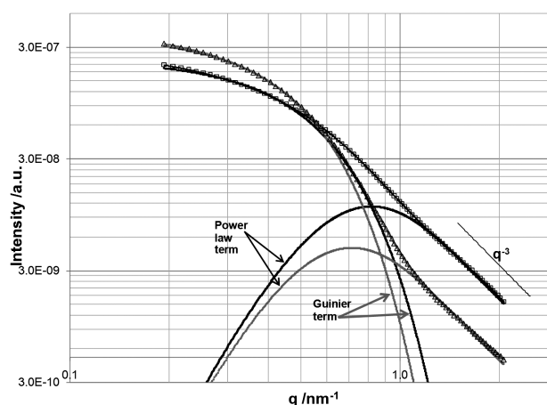
Figure 4: Measured SAXS profiles from FePt- (squares) and Fe 3 O 4 - (triangles) nanoparticles. The black and grey solid lines are the unified exponential power-law fits for FePt and Fe 3 O 4 , respectively, with the contributions from the Guinier and power-law terms. The q^{-3} line is shown to indicate -3 slope obtained from the fit.
