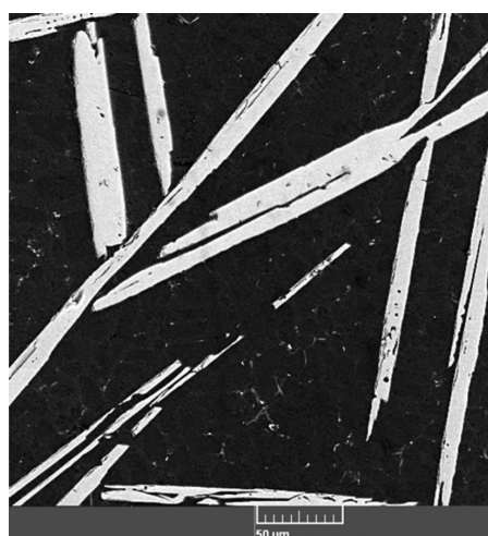
Figure 1: SEM micrograph of the as-cast Al-14Si-8Fe alloy containing large \beta -Al 5 FeSi plates (light) deteriorating the mechanical properties
