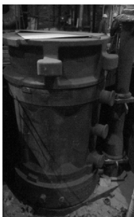
Figure 1: Comparison between the real and the CAD geometry of the casting system for a 90-ton ingot 2
