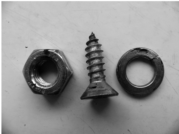
Figure 4: Corrosion-damaged structural components after cleaning with ultrasound
