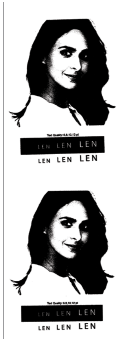
Slika 4: Vizualna primerjava izbranega elementa odtisa za vzorca BC papirja (levo) in BC-Š-3NCC (desno) Figure 4: Visual comparison of the selected printed element for a sample of BC paper (left) and BC-Š-3NCC (right)
