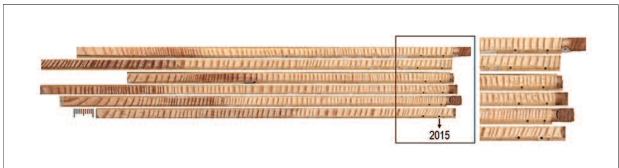
Figure 4. Increment cores of Pinus pinea polished and scanned at the resolution of 1200 dpi. Black dots indicate the tree rings dated 2010 (left) and 2015 (right). Intra-annual density fluctuations (IADFs) in tree ring 2015 cannot be clearly seen, the wood formed between March 2015 and the end of January 2016 would be considered as the annual ring for 2015. Wood produced between January and March 2015 would be ascribed to the 2014 increment (c.f. Figures 2 and 3).
