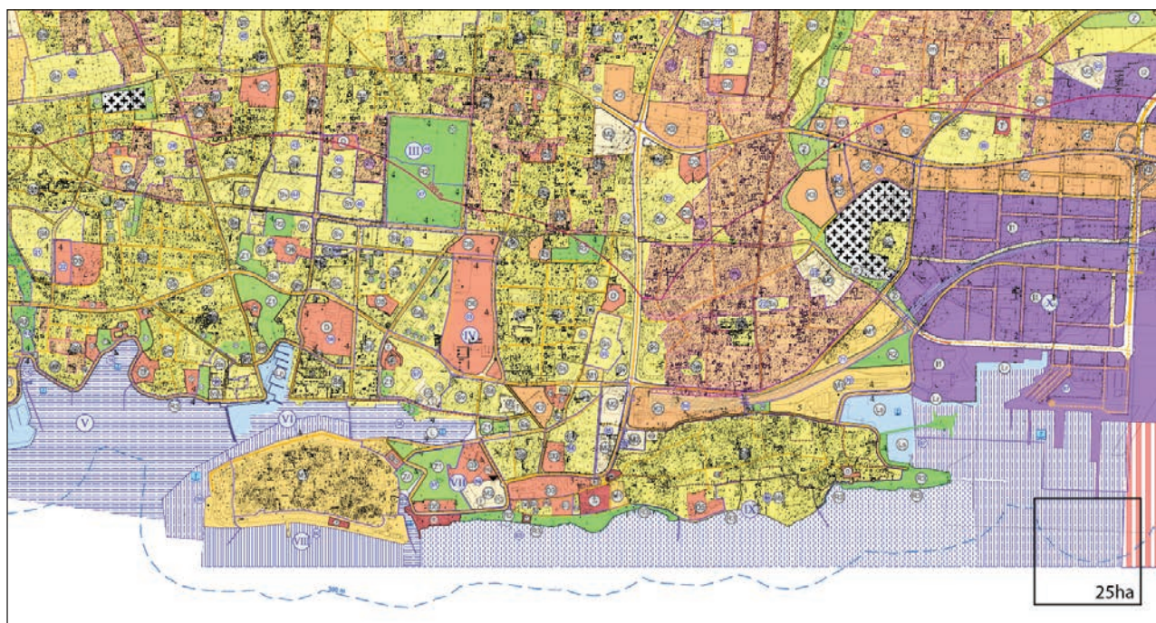
Figure 13: Zadar County Spatial Plan, map 5. Development and organization of the settlement – cut-out, amendments 2011. Legend: (S) residential, (M) mixed use, (K) business, (D) public, (T) tourist, (Z) green, (R) sport and recreation, (I) industrial (Gradsko vijeće Grada Zadra, 2004, www.grad-zadar.hr )
