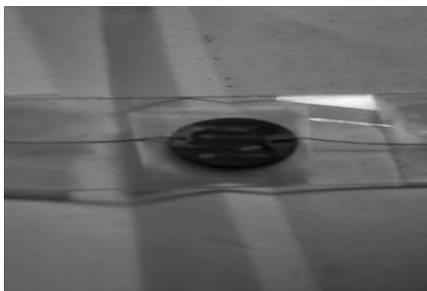
**Figure 7:** Photograph of developed humidity sensor based on the potash alum/fly ash composite
