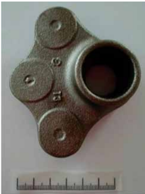
Figure 2. Shape of steering mechanism after the last hot forging operation
