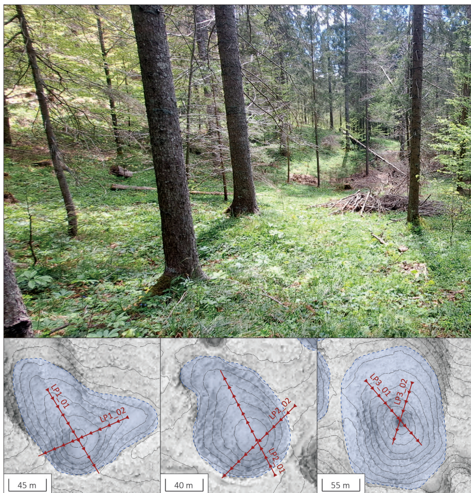
Figure 5: Elongated doline in Loški Potok (top) and maps of ERT profiles on LiDAR-derived visualisation with 2.5 m contour interval (bottom).
