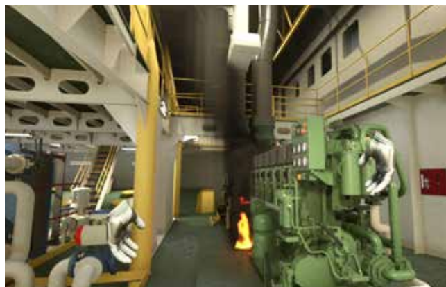
Figure 1 : VR-model of fire spreading in a ship engine room.
