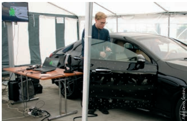
» 3D skeniranje s Shining 3D Einscan Pro 2X Plus
