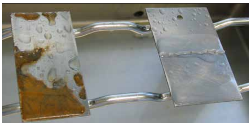
Hydrolubric VG 46 18PI163 (TOMA-DBP+NMP) Figure 3. Corrosion in the humid chamber after 24.5 h – mineral hydraulic oil vs. IL 18PI163
