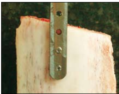
Figure 8. Plate mounted on a pig rib for the extraction test.
