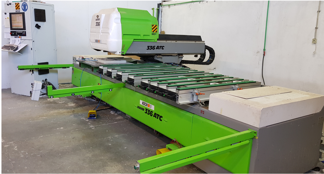
Figure 1.: Machining center Biesse Rover 336 ATC with four axes, two spindles and two tool magazines located at different sides of the working space.
