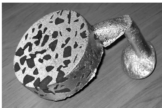
Figure 8: Casting made of AlSi10MgMn with remaining precursors
