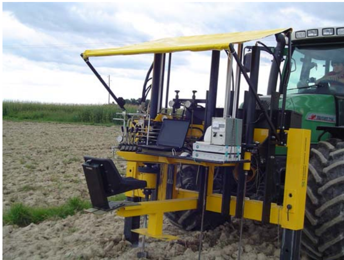
Slika 1: Naprava za določanje mehanskih lastnosti tal Figure 1: Device for acquisition mechanical properties of soil
