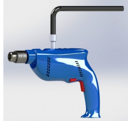
Fig. 3 A schema of drill made with internal gas cooling
