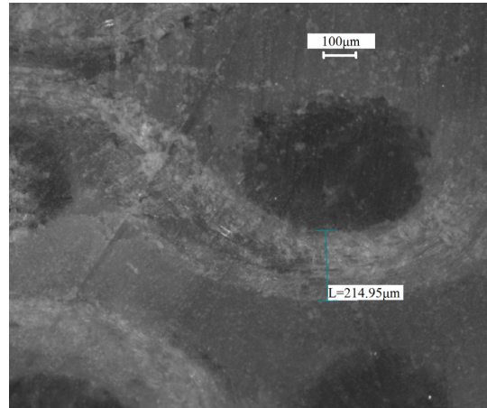
Fig. 14. Cross section of a weft yarn
