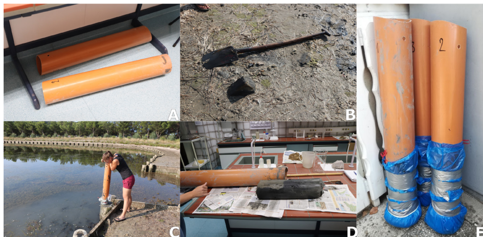
Figure 3: Soil sampling. A) Sewage pipes for taking soil samples; B) Spade for excavating pipes containing samples; C) Soil sampling; D) Extracting the sample from the pipe; E) Drying of soil samples (photos A–D: B. Repe; photo E: T. Pavlin).
