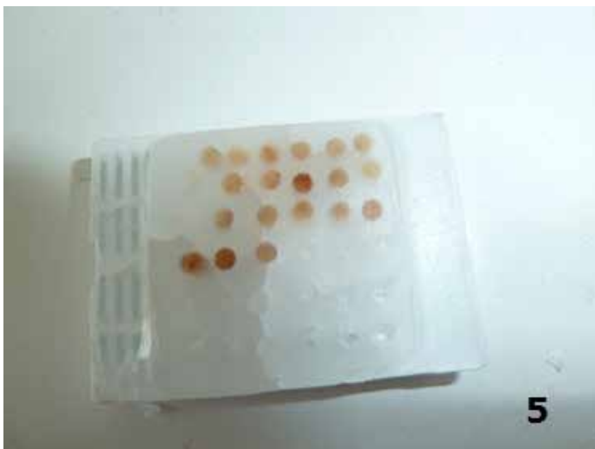
Figure 5. Cracked tissue array block after extensive and quick cooling.
