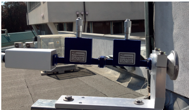
Figure 12: Waveguide attenuators for dynamic range determination
