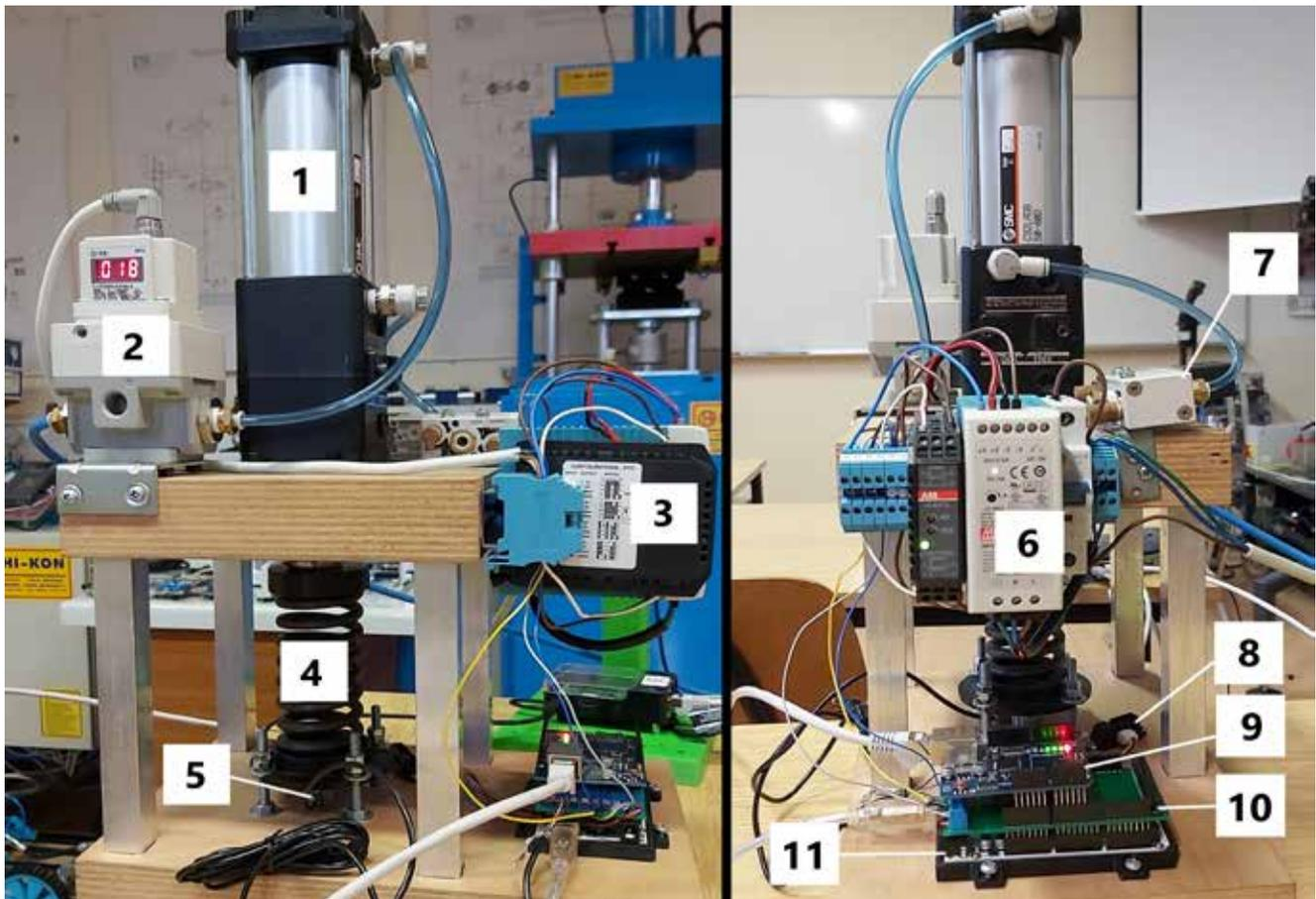
**Figure 1 :** Pneumatic press: 1-Pneumatic cylinder, 2- Proportional pressure-control valve, 3-Signal converter, 4-Spring, 5- Load cell, 6-Power supply, 7-Monostable valve, 8-Position sensor, 9-Arduino Ethernet shield, 10-Printed circuit board, 11-Arduino MEGA microcontroller
