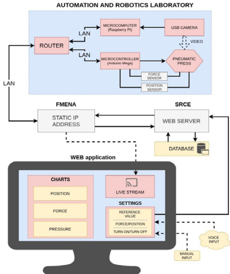
Figure 3 : Block diagram of the web-controlled system
