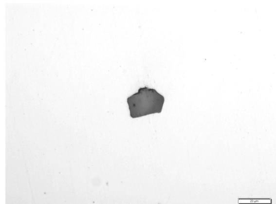
**Figure 15:** Non-metallic inclusions in the forged piece in Melt 3; magnified 330 times
