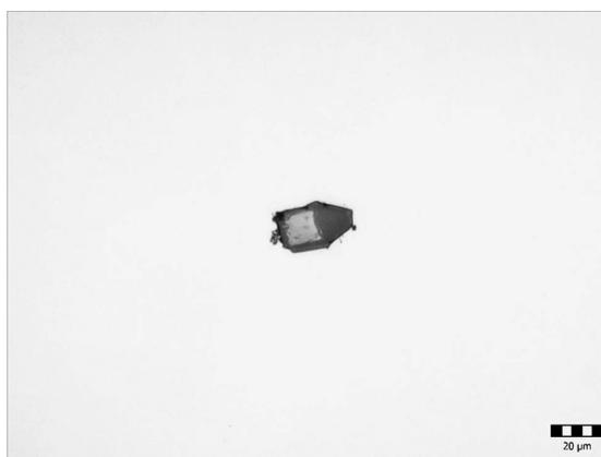
**Figure 10:** Non-metallic inclusions in the piece forged from Melt 2; magnified 330x
