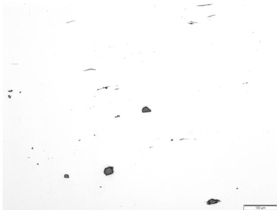
**Figure 14:** Non-metallic inclusions in the piece forged from Melt 3; magnified 65x
