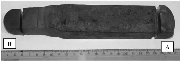
**Figure 15:** Forged sample after the final forging operation
